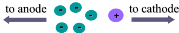
Figure 2 – In outer electric field the movement of a cation toward the cathode is retarded due to the ionic atmosphere
